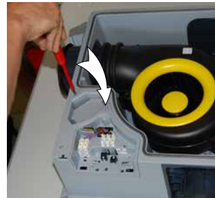
28. Fix the electrical case on the fan case (4 screws).
