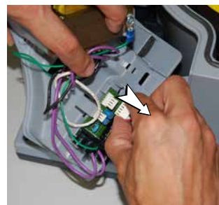
3. Unscrew (1 screw) and withdraw the trap door of the electrical case.
