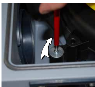
25. Fix the mototurbine (3 screws).
