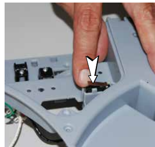
11. Place the switch of the new supply set. Keep the original position! (see picture 10).
