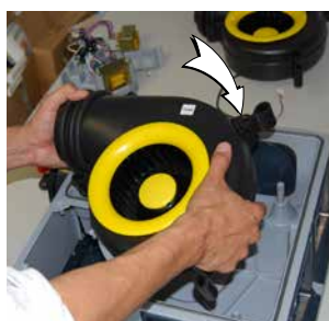
20. Place the new mototurbine. Make sure that the exhaust spigot is well engaged! (no space between mototurbine spigot and exhaust spigot).
