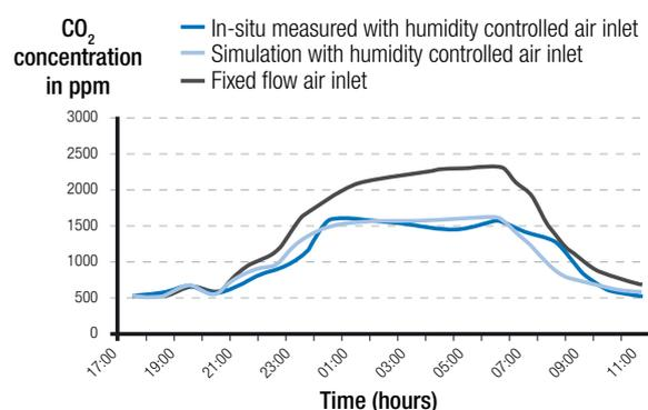
Figure 2: Overnight variation of CO<sub>2</sub> concentrations in a bedroom. Comparison of HC air inlet (measured and simulated) and fixed-flow air inlet (simulated).
