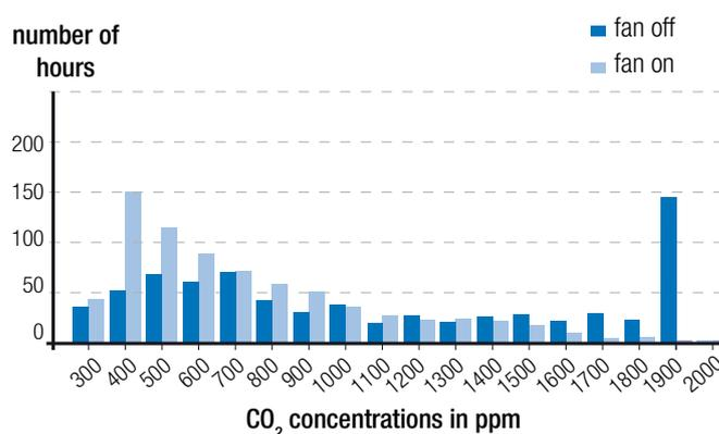
Figure 3: CO<sub>2</sub> concentrations with/without ventilation. Measurements for one month with fan off in a bedroom compared with fan-on for the rest of the heating season. 3 occupants in a bedroom.
