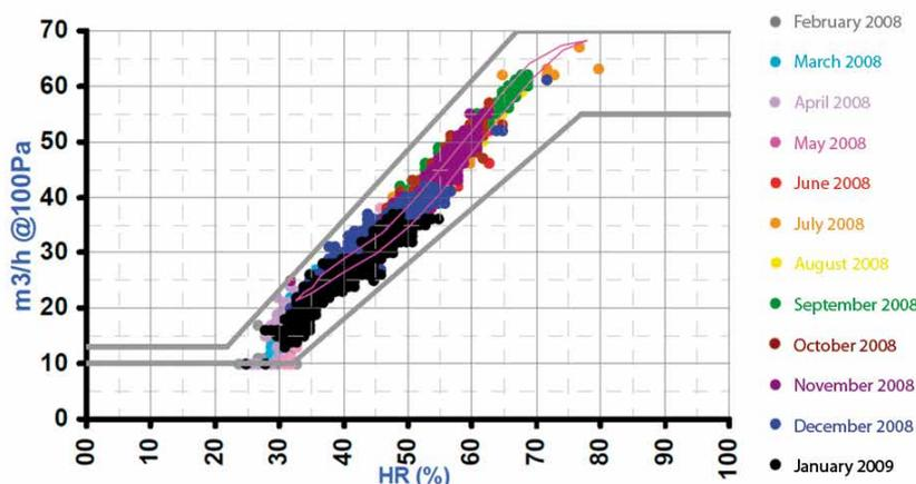
Figure 5: Airflow/RH behaviour of a humidity controlled extract unit in the kitchen. Pink curve = laboratory measurement. Grey lines = tolerance envelope. Dots points = measurements.
