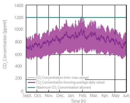
This study has also shown that, in real occupation conditions, Aereco Demand Controlled MEV system is an excellent way to stay below 1,200 ppm CO<sub>2</sub>, which guarantees an optimal Indoor Air Quality in the dwelling (graph n.3).
